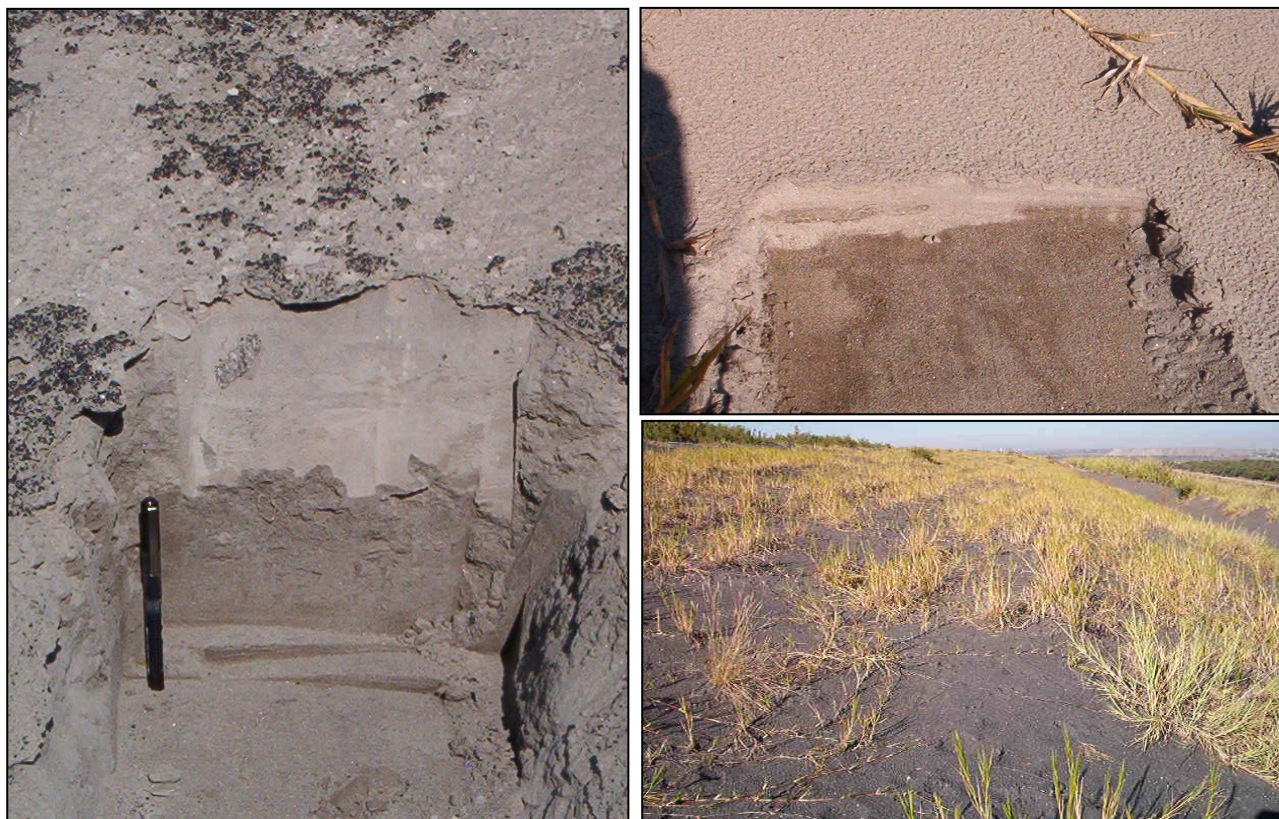
Figure 2 Platinum tailings material. Note the visual dry-out depth at field capacity on the tailing slope (left) and roadway (upper right). Natural vegetation establishment is an anomaly on this material and vegetation consistently experiences drought stress with slow rate of soil nutrient cycling
