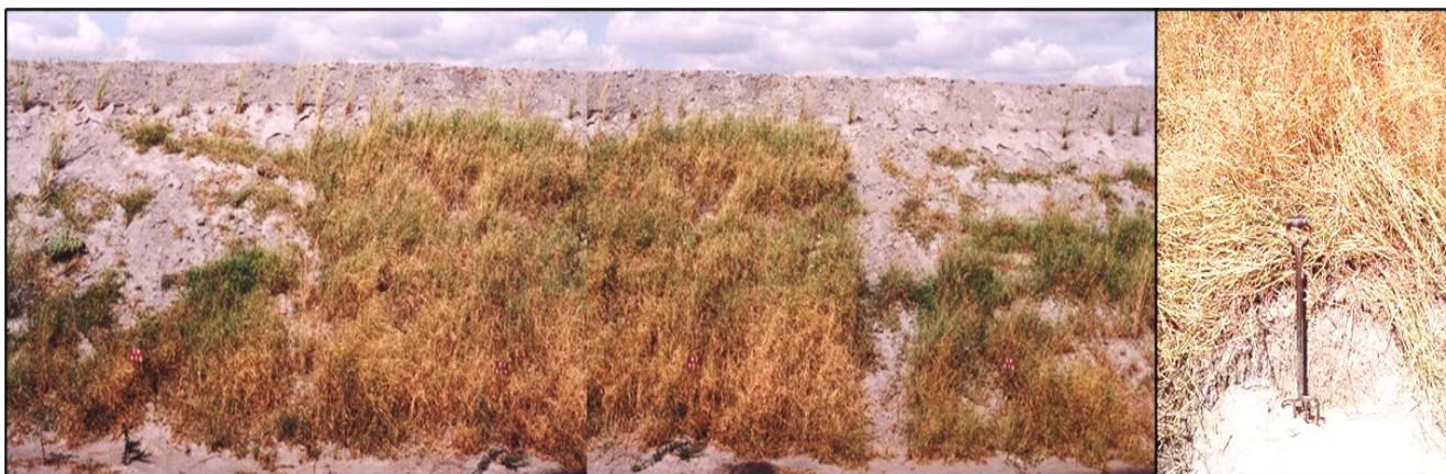
Figure 3 Visual representation of the rehabilitation trial on platinum tailings. Vegetation was successfully established and the maximum root depth of 0.8m was achieved for the best treatments (treated biosolid application and grass mulch covers)
